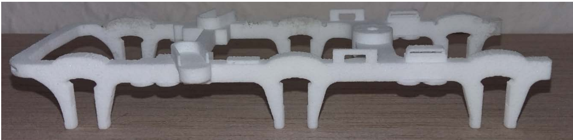
First sample in On3 scale from rapid prototype material.
