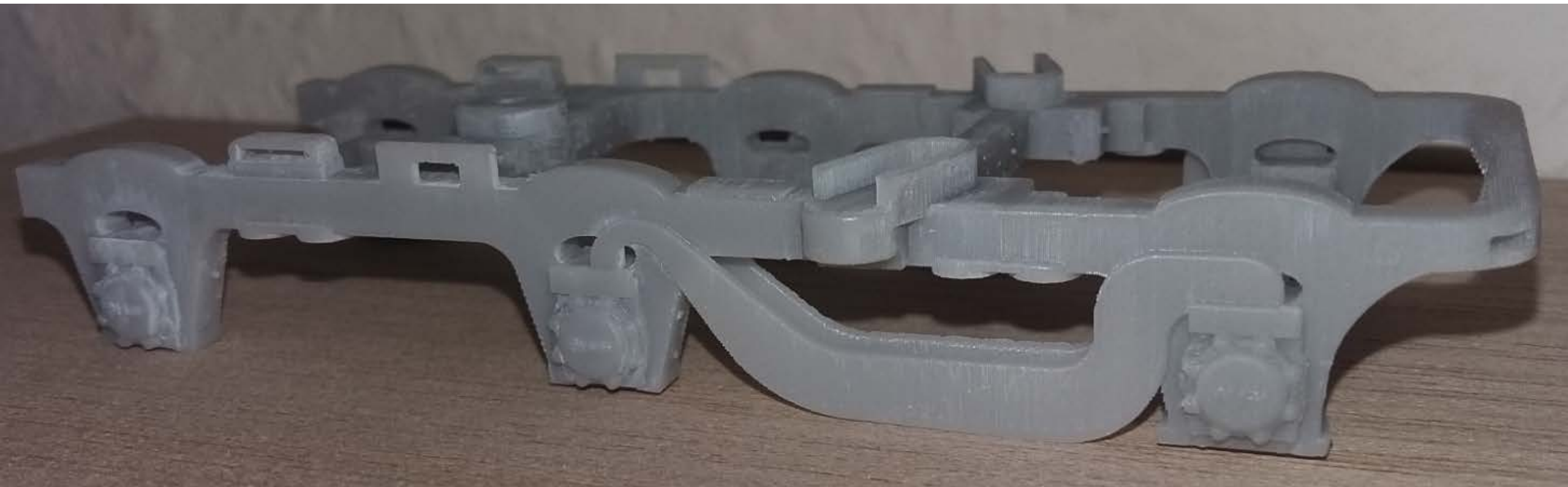
On3 Sample with Bolster and equalizer bar in different stage.
